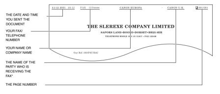
\* When using speed dialing, the top line also includes the name registered under the speed dialing button or code you entered.
